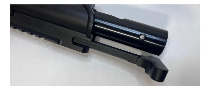
**04** / Once the charging handle is removed from the upper receiver, pull it back, then tilt it into alignment with the barrel and finally remove it.
